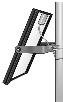
*Solar panels are convenient charging sources for applications where ac power is not available, unreliable, or expensive. The SP10 sources sufficient current for many of our systems.*
